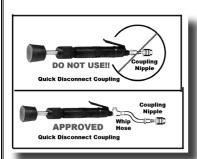
Attachment of a quick-disconnect air coupling directly to the inlet threads of a percussion tool can cause wear and failure of the coupling. Should the coupling fail, severe injury can result from the hose end violently whipping about. If a quick-disconnect air coupling is used, separate the coupling from the tool with a whip hose (1.5 feet minimum). Only use
